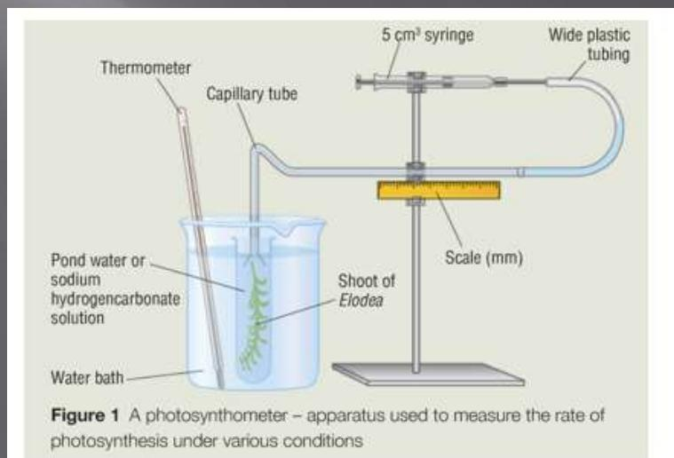
**Figure 1** A photosynthometer – apparatus used to measure the rate of photosynthesis under various conditions
